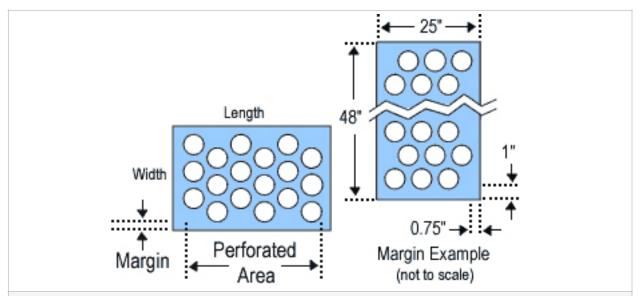
Tolerances There are tolerances on quantity, shearing, gcircle shearing, flatness, thickness and squareness, for perforated products. If you do not specify a specific tolerance, the standard tolerance applies. Tolerances can be specified on the perforated round hole pattern quote form.
