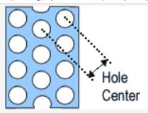
Open Area Perforated sheets contain holes and material. Open area is the total area of the holes divided by the total area of the sheet and is expressed as a percent. In other words, open area describes how much of a sheet is occupied by holes. If a perforated sheet has 60 percent open area, then 60 percent of the sheet is holes and 40 percent is material. Note:
