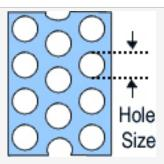
Hole Center Hole Center is the distance from the center of one hole to the center of the nearest hole in the next adjoining row. Hole center is one of two measures of perforation spacing. The other is open area. Because hole center and open area measure essentially the same property (perforation spacing), you need specify only one or the other, not both.
