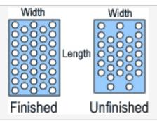
Length and Width Length is the overall measurement of the long side of the sheet; width is the overall measurement of the short side of the sheet. Note that mill tolerances for length and width apply to stock sheets unless otherwise specified. If you have a stock sheet cut-to-size, cut-tolerances apply. To specify other than standard tolerances, please use the perforated round hole pattern quote form to specify the required tolerances.
