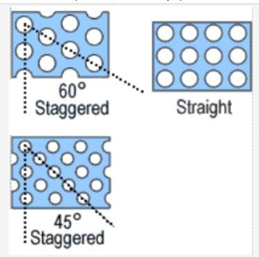
Hole Size Hole size is the diameter of the perforation. YUNHAO carries a wide range of round hole sizes (from 0.020 to 1 inch) and can special order any hole size required as long as it meets minimum hole size requirements.
